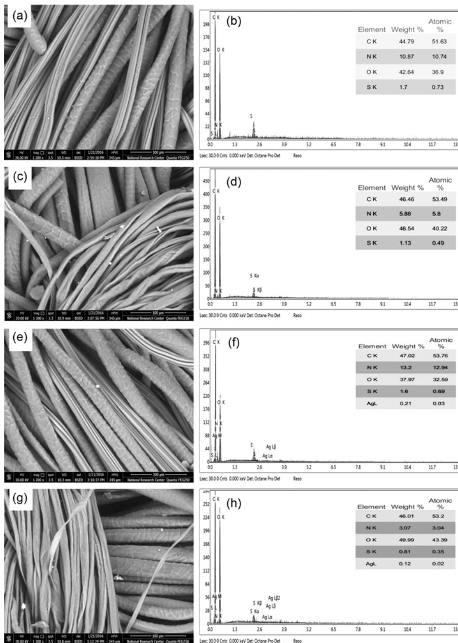
Figure 2. SEM and EDX of printed viscose/wool and cotton/wool fabrics (a,b) and (c,d) respectively. Printed viscose/wool and cotton/wool in presence of AgNPs (e,f) and (g,h) respectively.
