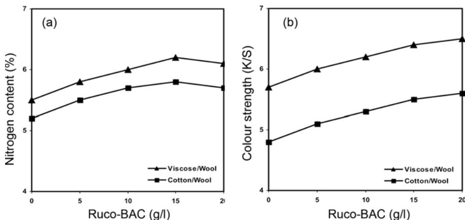
**Figure 4.** Effect of post-treatment of the printed fabric samples with Ruco<sup>®</sup>-BAC on nitrogen content (%) and colour strength (*K/S*) values.
