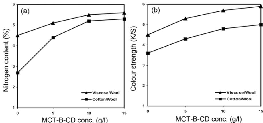
**Figure 3.** Effect of MCT- $\beta$ -CD concentration on the nitrogen content (%) and extent of post reactive printing (*K/S*) of the treated cellulose/wool blended fabrics.
