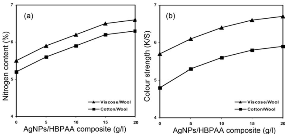
**Figure 5.** Effect of post-treatment of the printed fabric samples with AgNPs/HBPAA composite on nitrogen content (%) and colour strength (*K/S*) values.
